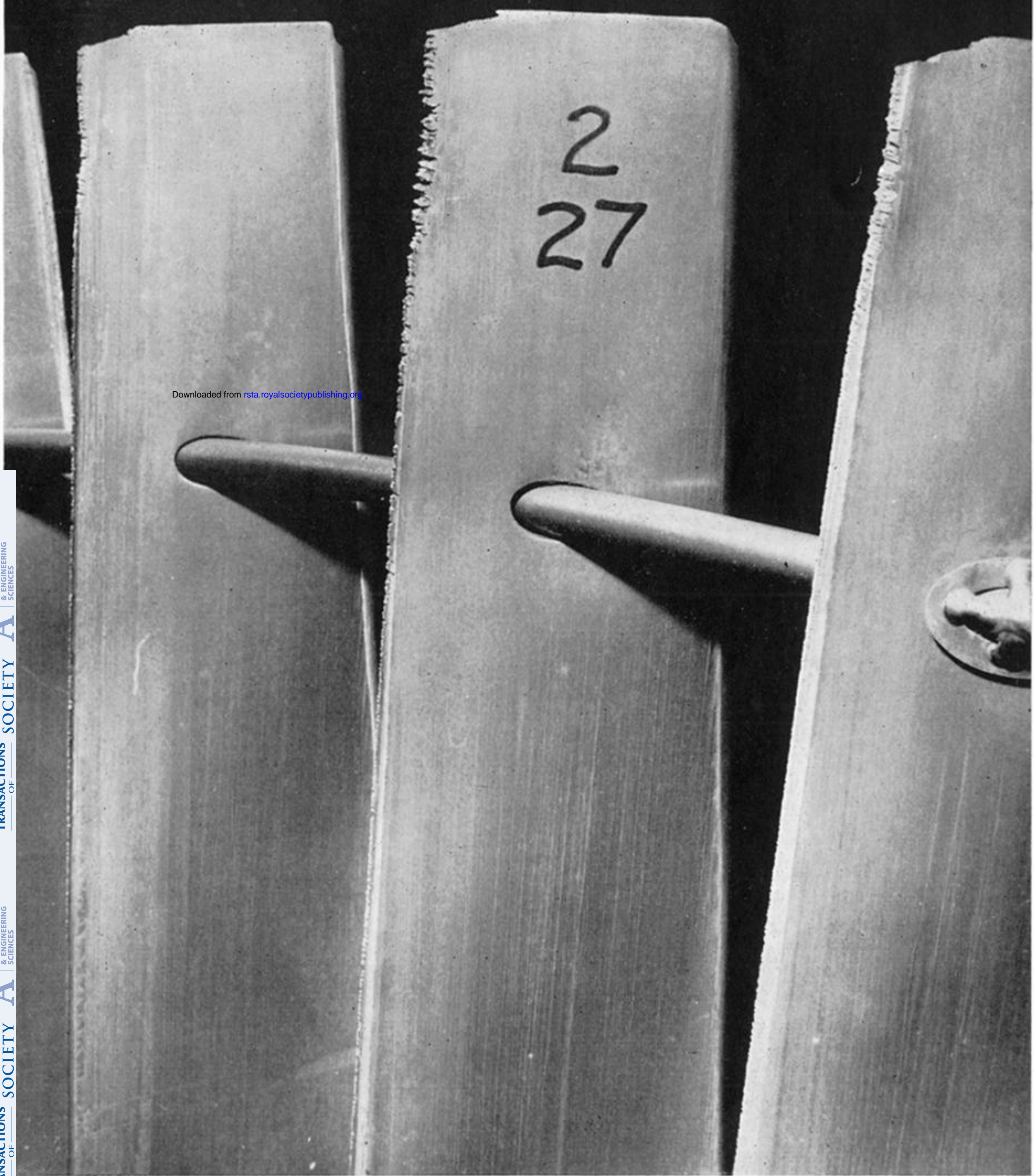
FIGURE 6. The erosion damage on the 36 in. blading run in connexion with the wide closely set diaphragm of figure 4 opposite.
