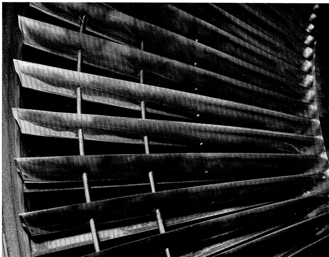
FIGURE 3. Tangential erosion of stainless iron blades behind the cobalt alloy shields. The middle blades are of stainless iron, those on either hand of manganese nickel steel (0.8% Mn, 0.9% Ni) hard chromium plated to a thickness of 0.001 in.
