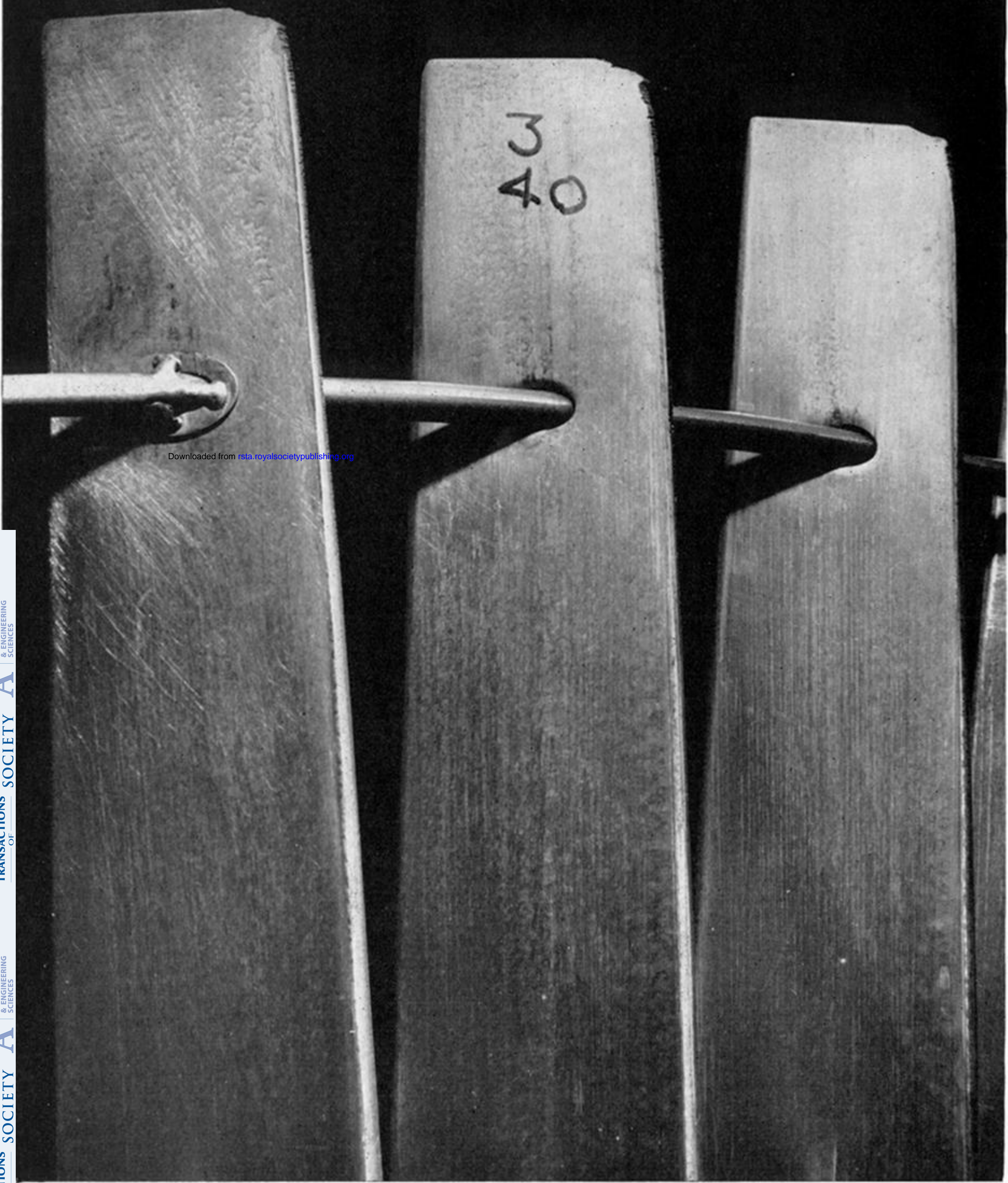
FIGURE 7. The greatly reduced damage resulting from the use of the narrow diaphragm set farther back from the running blades as in figure 5.
