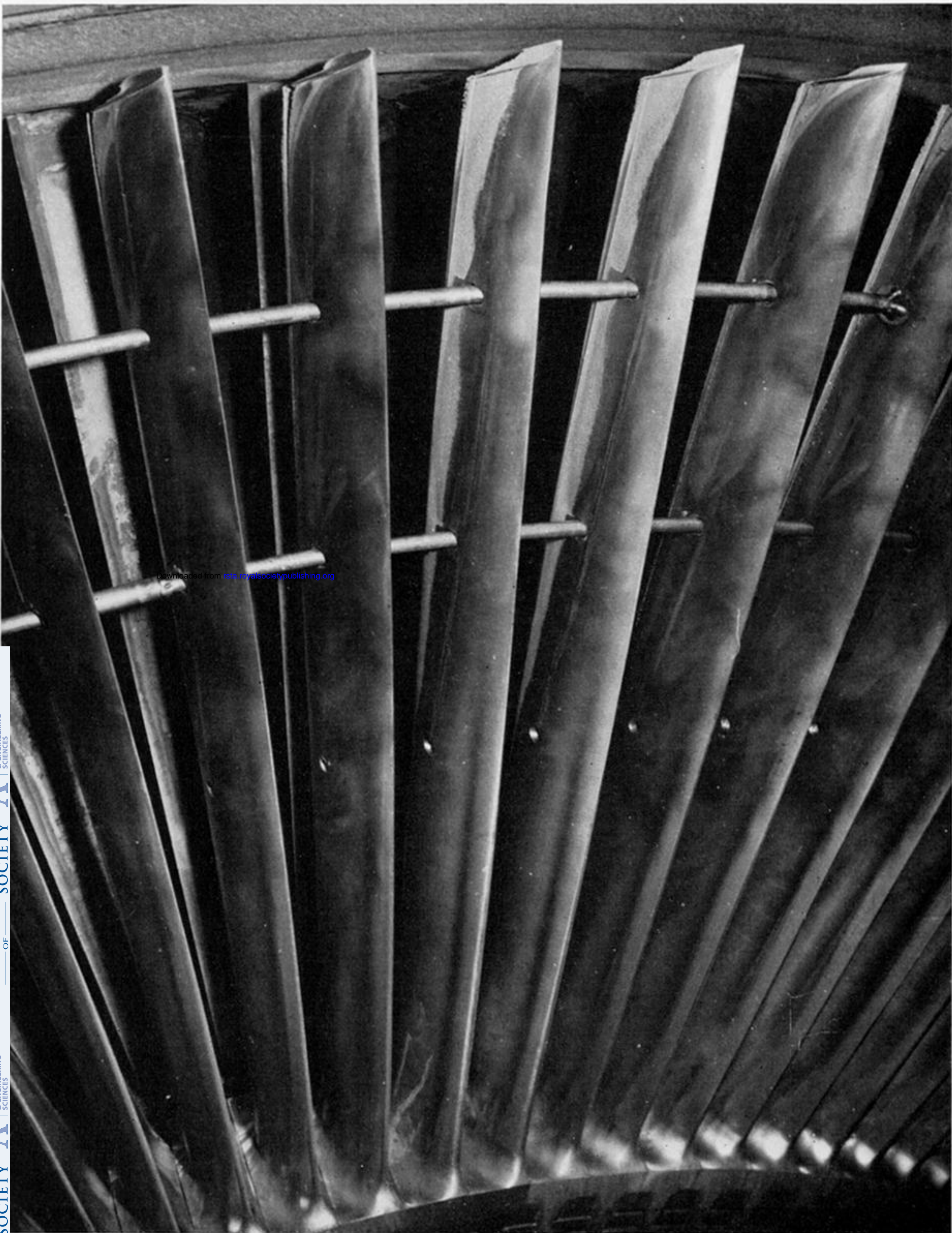
FIGURE 3. Tangential erosion of stainless iron blades behind the cobalt alloy shields. The middle blades are of stainless iron, those on either hand of manganese nickel steel (0.8 % Mn, 0.9 % Ni) hard chromium plated to a thickness of 0.001 in.
