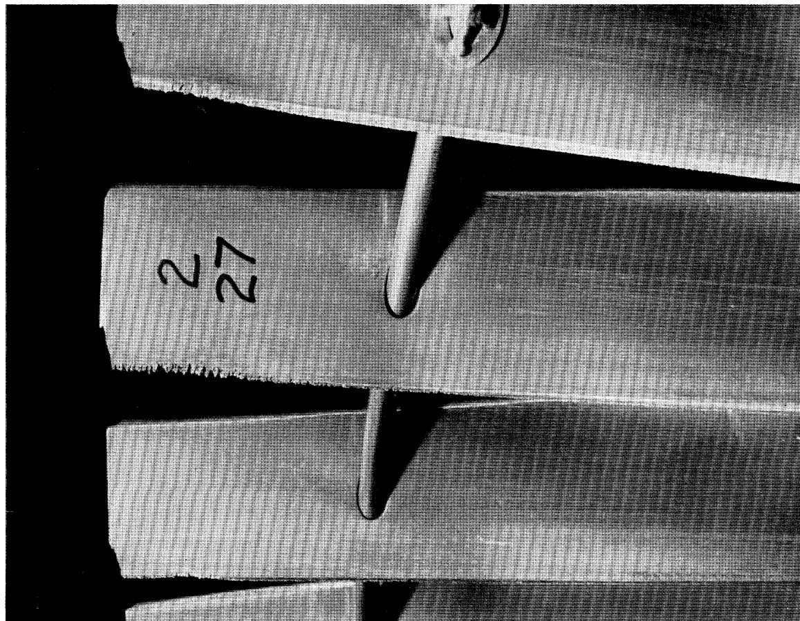
FIGURE 6. The erosion damage on the 36 in. blading run in connexion with the wide closely set diaphragm of figure 4 opposite.
